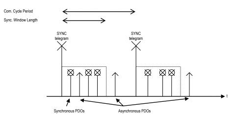
The synchronous PDOs are transmitted directly after the synchronization telegram in the defined time slot **Sync. Window Length** [µsec]. If Com. Cycle Period and Sync. window length are 0, then no synchronization telegrams are transmitted.
